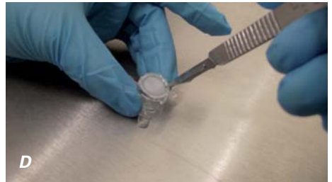
Figure 4. Removal of alvetex ® disc from well-insert. Unclip the base of the well insert all the way around (a.), and pull down to release the disc (b.). Alternatively the disc can be cut out by holding the well insert upright (c.) or upside down (d.)
