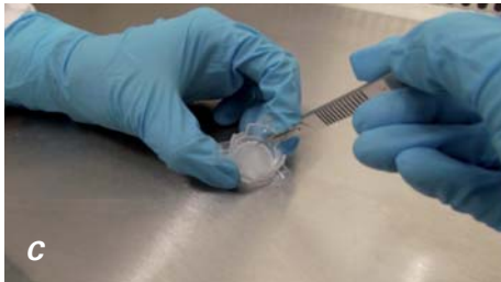
Figure 4. Removal of alvetex ® disc from well-insert. Unclip the base of the well insert all the way around (a.), and pull down to release the disc (b.). Alternatively the disc can be cut out by holding the well insert upright (c.) or upside down (d.)
